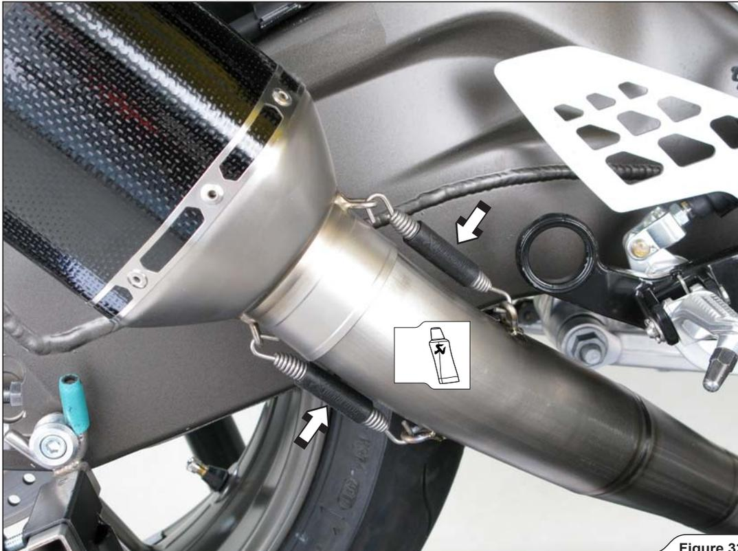
16. Align the muffler in respect to the motorcycle and tighten the muffler clamp to the bracket, using Akrapovič bolt, washers, and nut as shown (Figure 33).
